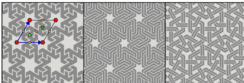
Figure 18. Three ornaments of the group p6 . The symmetry operations are superimposed on the pattern on the left. Translation vectors and thin black lines define the unit cell. Red hexagons are the sixfold-rotation axes. Threefold-rotation axes are represented as green triangles. Yellow diamonds indicate the twofold-rotation axes.
